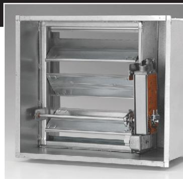
**Figure 4, Ruskin FSD60FA-BAL. Corridor fire & smoke & balancing damper with 3-position FSAF24-BAL actuator.**
